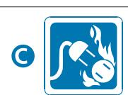
C. Use on electrical equipment and wiring.
